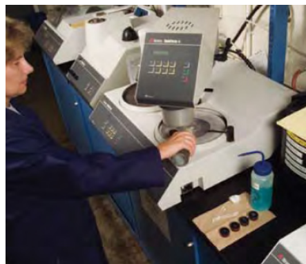
Metallographic specimens are bisected, cleaned, hot mounted, ground, and polished.
