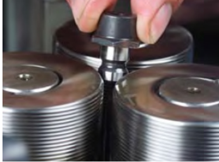
A vertical three die process is often used when tight concentricity is important.
