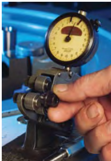
Aerospace industry specifications require that indicating type gauges be used to measure threads.
