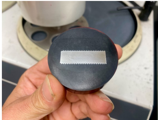
After polishing to a 3 micron finish, the specimens are etched to reveal the microstructure.
