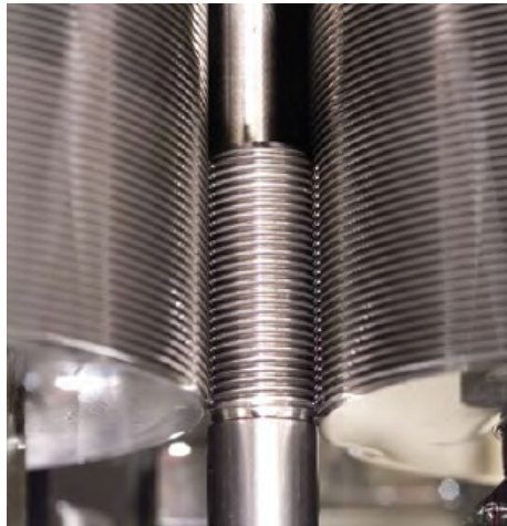
A horizontal two die process is suitable for both infeed and thru-feed rolling.
