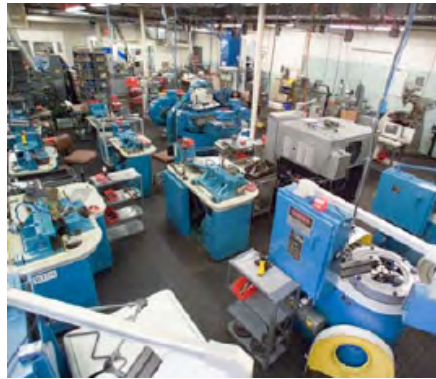
A variety of machine types and sizes to roll threads
