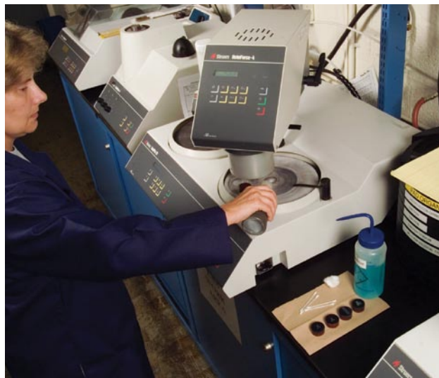
Above: Metallographic thread specimens must be bi-sectioned, cleaned, hot mounted, ground, polished, and etched prior to inspection.
